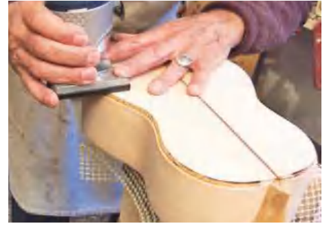
STEP 37. Cutting the binding and purfling channels
